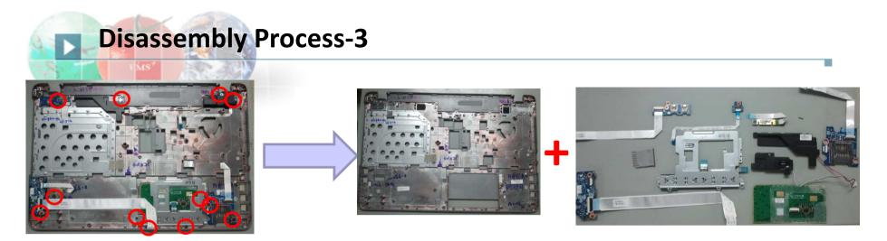
Loose the screw of the speaker ,power board, function board, touchpad module, FPR, SD board ,and USB board then take off them.
